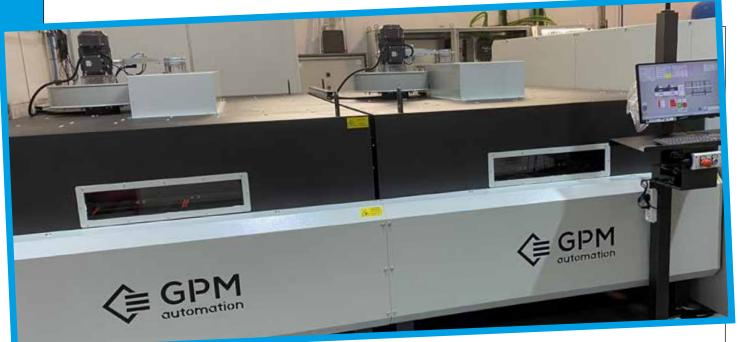
that all types of glass and interlayers are processed using the most efficient parameters. The newly installed press also represents a significant technological advancement. Powered by servo motors on an electric axis and guided by specialised software, the press continuously monitors the flatness of the top roll via servo-drives. This ensures precise and uniform pressure distribution across all glass sizes, thereby eliminating the need to centre glass pieces on the press bed. The system's
