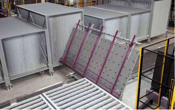
into existing production lines quickly without a large space requirement. Tilt tables and / or transport fields can be replaced by robots. The overall integration into the existing processes is important, e.g. integrating a downstream rotary platform to ensure a continuous workflow.
