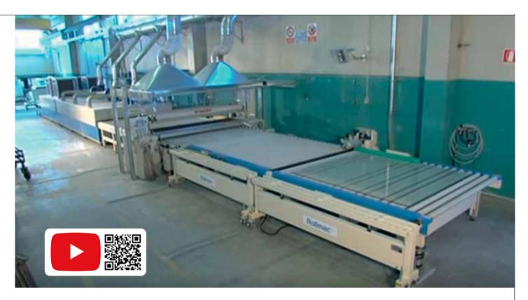
trol panel. Worthy of note, the machine control PLC enables a frame setting with four parallel bands of varying widths - all on a single sheet.
