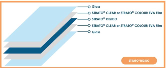
is available in different formats and widths. STRA-TO® RIGIDO is also available in different thicknesses and roll lengths.
