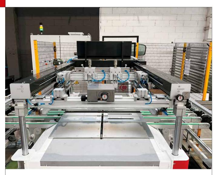
pressure and speed to frame regulation up to peel off height. The Compact 4C allows for the processing of big, symmetrical batches in reduced times - ensuring, for example, 550 pcs/h for glass with dimensions of 1144x692 mm. Printing precision between every piece is +/- 0,08 mm, which gives standard quality to the final product. As with all Cugher machines, this one can be integrated in line with innovative vision systems for quality control - both for glass and printing.
