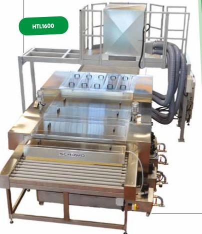
chine. The model offers an excellent quality/price ratio. TOP is designed for glass with heights ranging from 1600 to 3300 mm, with a thickness of up to 20 mm. Here the machine features a robust structure made entirely of stainless steel,
