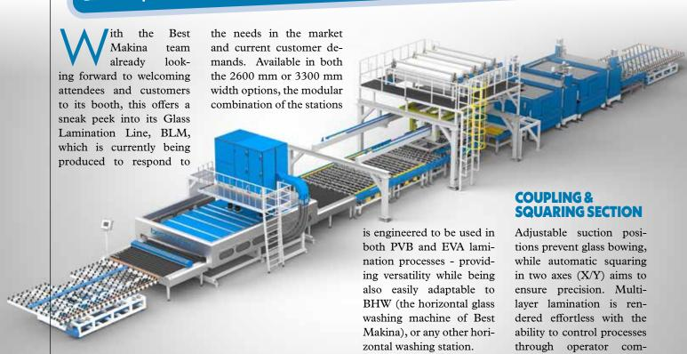
mands or predefined recipes. The automatic PVB feeding with length control and cutting systems ensure a seamless process. The technology of non-marking rollers facilitates the movement of glass without leaving any surface marks - ensuring a smoother and cleaner workflow.
