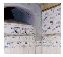
The preheating phase itself lasts about ten days and is required to gradually bring the furnace up to the temperature that will allow it to operate at full capacity, which is 1350/1400°C. To progressively reach this temperature only scrap glass is introduced - that is, a part of the vitrifiable composition which, once melted, will be transformed into liquid glass, given that it has a lower melting temperature.
