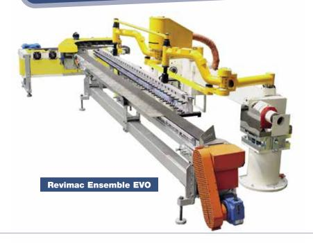
Revimac Ensemble Evo offers a stable system that's both synchronised and harmonious - combining the ware transfer triple belt XHS900, the cross conveyors RC900 (without cooling system) and the RSS100 lehr loader (stacker). Already chosen by some of today's largest groups and glass plants, the consolidated technology is often preferred when fulfilling a need for very stable container handling.
