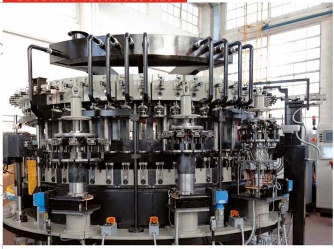
function as well in case the customer needs to process stemware pieces made of just one piece and made in a dedicated pressblow machine. In this case the SA model is converted into ST - also available in 42, 48 and 60 stations according to the productivity needed by glass factories.
