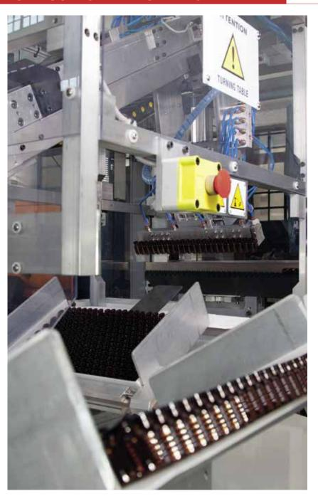
able to be connected with the automatic loader supplied by OCMI, now available in the new version picking the single tube from the packed bundle.
