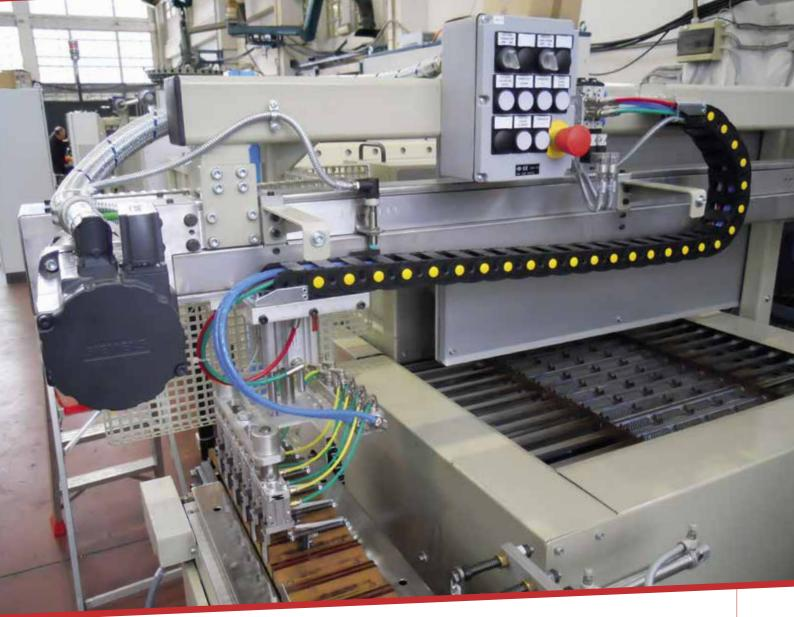
formed by way of three dedicated stations, each respectively dedicated to roughing and shoulder preparation, pre-finishing and finishing. The stations follow rotation of the upper chucks via rotating bearings that have been mounted upon forming heads such that no manual alignment with the chucks is necessitated. All three stations are removable, thereby facilitating easy maintenance and job-change operation on the part of the operator.
