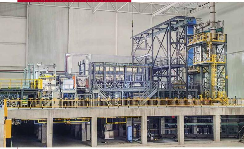
TPD where electrical components attaining high fusion energy percentages obtain a much reduced gas consumption. Consequently, a very low CO2 footprint that can maintain a high flexibility with production quality guaranteed by cross-fired furnaces with oxygas combustion.
