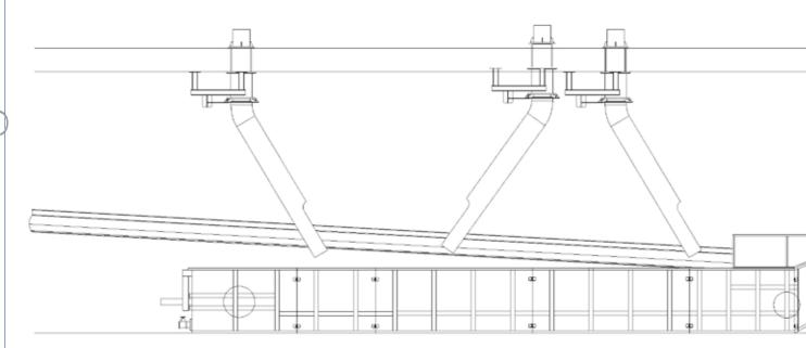
waste glass from furnaces and forming machines is the Scraper Conveyor. It cools and granulates the hot glass so it can be reintroduced into the production flow. This is achieved thanks to a continuous supply of water by which thermal energy from the glass is absorbed.
