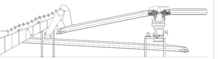
resistant dragging rods transports the glass while facilitating contact with the water. The granulation process occurs due to the thermal shock resulting from contact with the lower temperature water.
