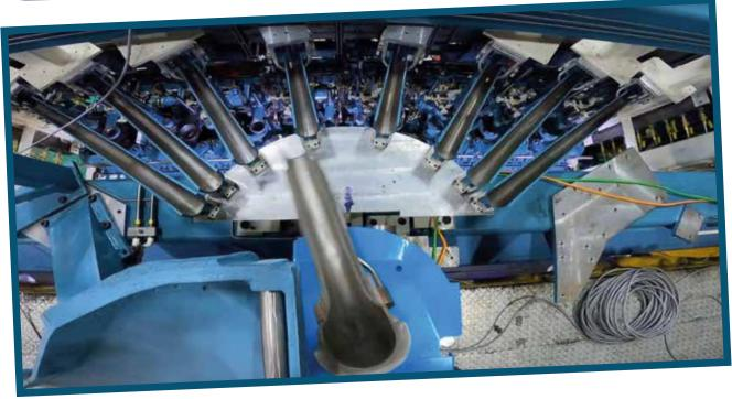
nism, a servo funnel mechanism, baffle and blow head, a servo take out mechanism using the new servo motor technology and a new mould cooling system.
