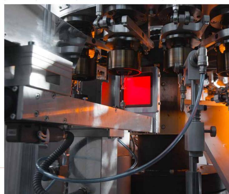
connected with the OCMI R-ATL4 loader, an anthropomorphic last generation multi-axes robot which allows for single tube picking from a muti-bundle high capacity magazine. This combination ensures maximum flexibility and minimizes contact/friction between tubes, which will effectively troubleshoot even minor cosmetic defects on finished products.
