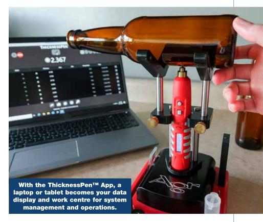
in real-time and easily captured for data processing. In addition, all basic ThicknessPen<sup>TM</sup> management functions can be conducted with the Appincluding calibration, unit and mode selection. With the App, system software never goes out of date and upgrades are easily managed.
