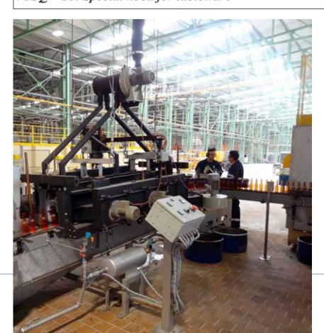
Notably, the geometry of the new convergent/divergent interior duct ensures better temperature control, distribution and uniformity of the coating film across the entire bottle diameter.
