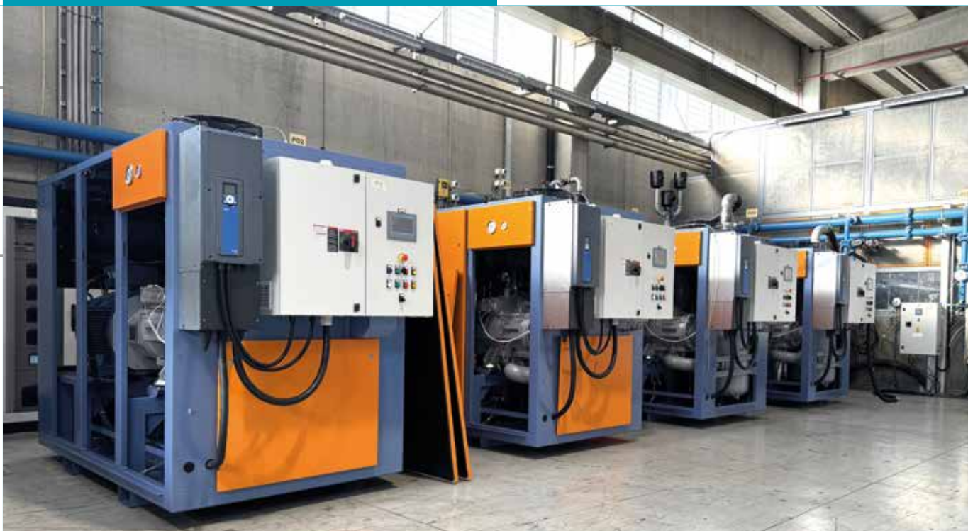
Four UV50 vacuum pumps being tested at Pneumofore for 12,000 m 3 /h capacity, November 2024
