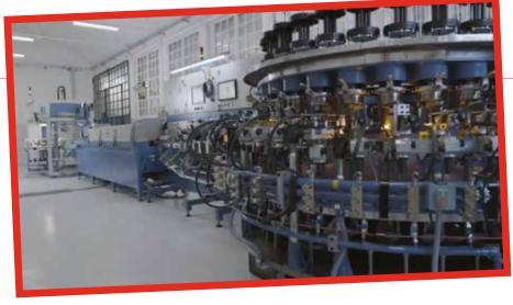
sional control, allowing operators to monitor all spindle dimensions while obtaining total length values on the same panel. A report with rejection statistics based upon different defects can also be generated.
