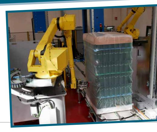
letizing. Manual film removal involves risks that originate from use by plant personnel of both cutting tools and ladders, passage on handling conveyors and the potential for items falling from the load unit. As such, installing EASYROCK at the infeed of depalletizing lines will greatly increase the overall safety of the working environment, as well as boosting line efficiency and providing maximum application flexibility.
