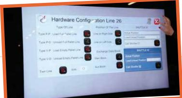
A new unique design solution introduced to the market just recently, ADVANCED CONTAINER HANDLING's Totem Glass Supervision System facilitates and coordinates management and handling operations and has both customized graphics and visualization for the cold-end.
