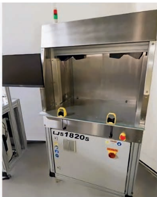
LJS1820S Manual 3D Static Measurement System (surface defects)
