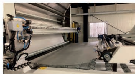
AUTOMATIC PVB FEEDING AND APPLICATION
