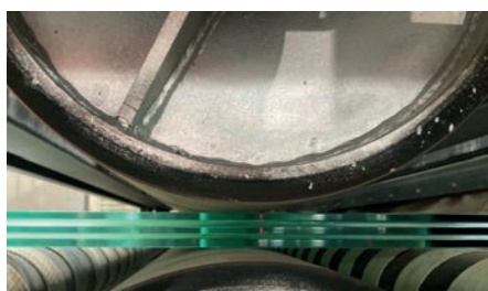
Laminated glass lines with electric press with servo drives, forced air convection ovens, fully automatic PVB application, cutting and trimming
