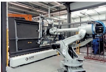
Robot and conveyors for IG line unloading
