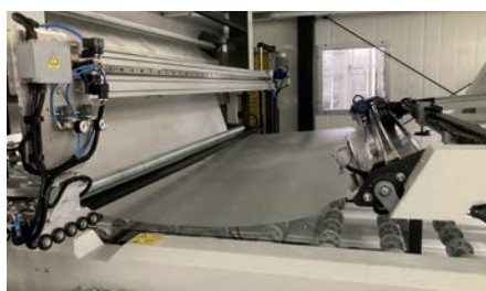
Laminated glass lines with electric press with servo drives, forced air convection ovens, fully automatic PVB application, cutting and trimming
