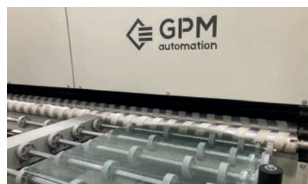
Laminated glass lines with electric press with servo drives, forced air convection ovens, fully automatic PVB application, cutting and trimming
