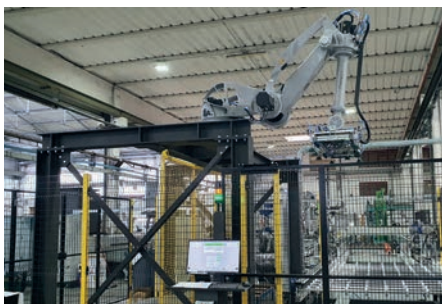
Robot and conveyors for double edger loading/unloading
