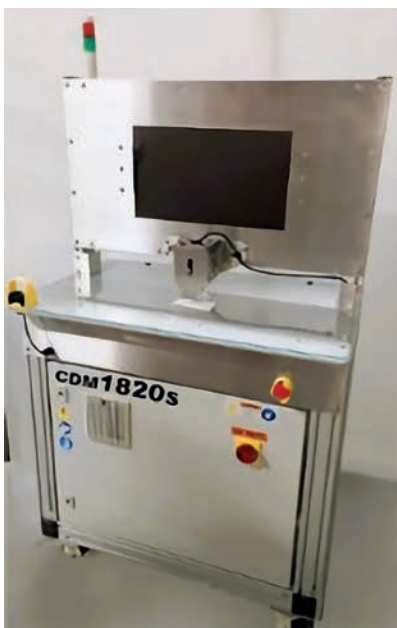
CDM1820S Confocal Differential Static Measurement System (material thickness)
