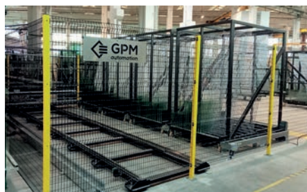
Harp racks and shuttle for IG line loading
