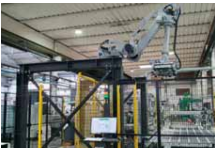
Robot and conveyors for double edger loading/unloading
