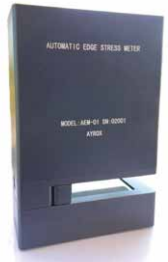
AEM of for automatic edge stress measurement
