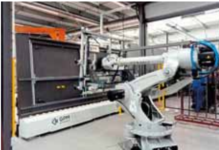
Robot and conveyors for IG line unloading
