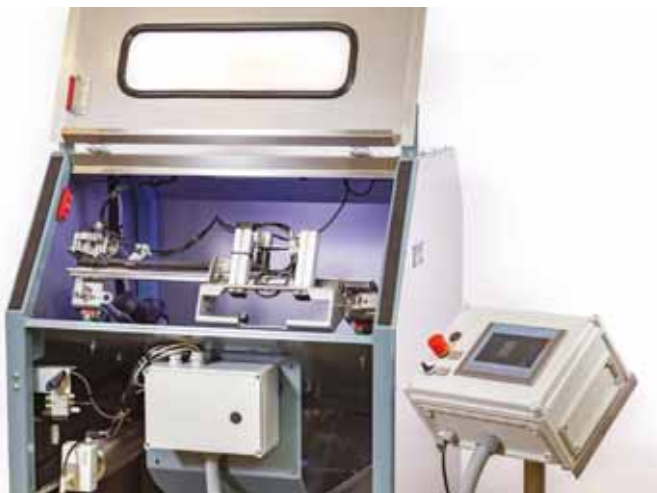
Automatic pummel tester according to EN 14449 and ASTM C1908
