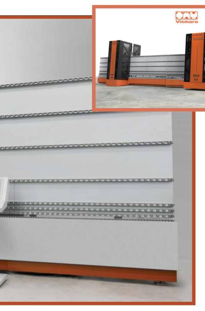
glass, for the production of doors and shower cubicles. OMV's product range for these demands includes lines made up of single machines, or single machines that carry out both types of processing (drilling and milling), as well as user-friendly machines and more performing machinery with tool storage (from 8+8 to 20+20 positions) and automatic tool changeover.
