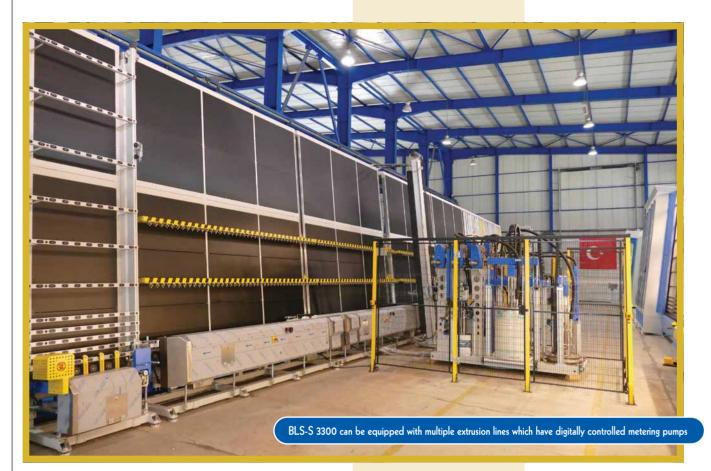
est Makina, global supplier of insulated glass production machines. is further strengthening its position in the IG machinery sector with a 3,300x6,000mm size complete insulated glass production line with automatic gass filling. With this new machine, the production of extra-height units is carried out by means of unique and flexible solutions which have been engineered in-house, facilitaing controls.
