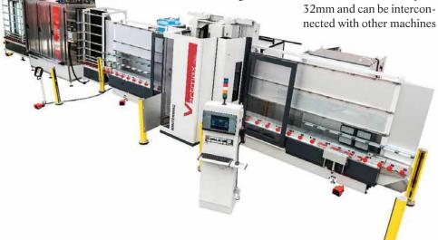
in the same line, allowing the processing speed and the machine opening to be managed in accordance with the thickness of the sheet of glass in question. High-capacity independent water tanks for each washing section reduce the need to change water frequently. Aqua washers can work on three shifts, with glass feed speeds up to 7 metres. It is also possible to arrange the processing direction, from right to left and from left to right.
