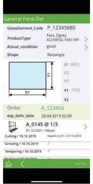
In future, operators will no longer have to rely on local data access at the control panel. Instead, they will be able to perform such tasks as triggering a new order for damaged glass, determining where a glass rack has been parked, retrieving maintenance information, reporting a malfunction, or re-ordering supplies — all using an app developed by HEGLA New Technology.
