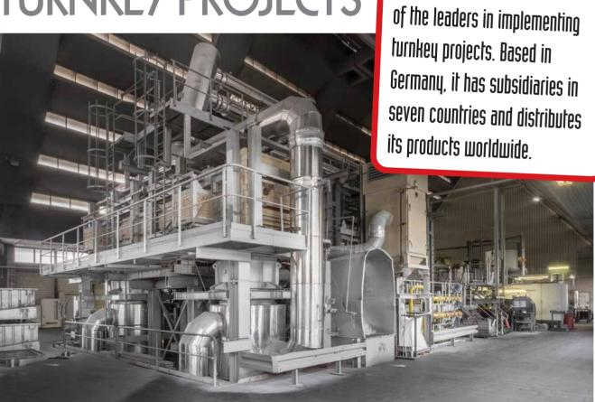
t its location in Plößberg, Germany, HORN Glass Industries AG plans and makes glass melting technology and turnkey projects for the float and container glass industry. The company's high-performance glass melting furnaces and turnkey projects are installed at glass manu-
