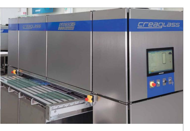
mented at any time on the basis of particular production and space requirements, thereby ensuring a high level of customisation. System Digital guarantees the quality of the printing, offering all the phases necessary in the decoration process in a compact solution composed of independent two point five metre modules.
