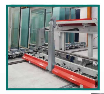
for those looking not only for space saving, safety and automation, but also top production flexibility, given that they can load several cutting lines simultaneously.
