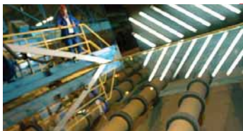
AGC Glass Europe - Moustier Plant: optical quality control of the continuous glass ribbon. Photographer: Jean-Michel Byl - © AGC Glass Europe
