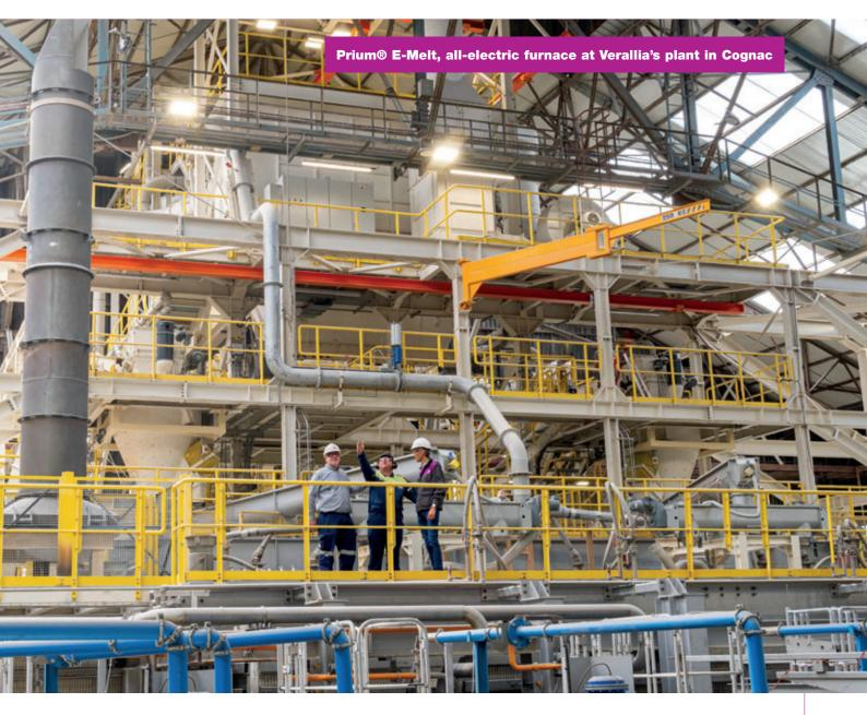
With a daily capacity of 180 tonnes, equivalent to 300,000 bottles, it reduces CO2 emissions by 60 percent compared to a traditional gas furnace. With the contract for the first furnace signed in September 2022, pre-engineering and design work started immediately. Construction occurred throughout 2023, with heat-up in March of 2024. The Prium® E-Melt furnace entered production at nominal design loads in April 2024.
