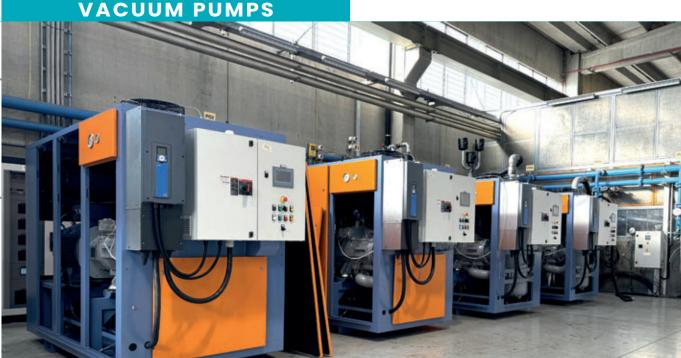
Four UV50 vacuum pumps being tested at Pneumofore for 12,000 m<sup>3</sup>/h capacity, November 2024
