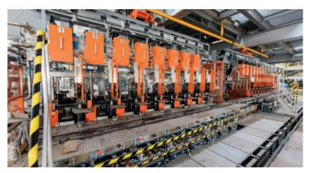
iner Glass is currently investing in a new greenfield container glass plant in Lommel, Belgium, with construction work now underway. The project in Lommel involves building a new, state-of-the-art container glass production facility. The site will host two furnaces, with a production capacity 650 tonnes per day. Each furnace will feed four production lines consisting of two 8+8 triple gob tandem machines and two 10+10 triple gob tandem machines.
