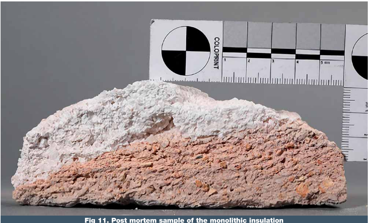
Fig 11. Post mortem sample of the monolithic insulation
