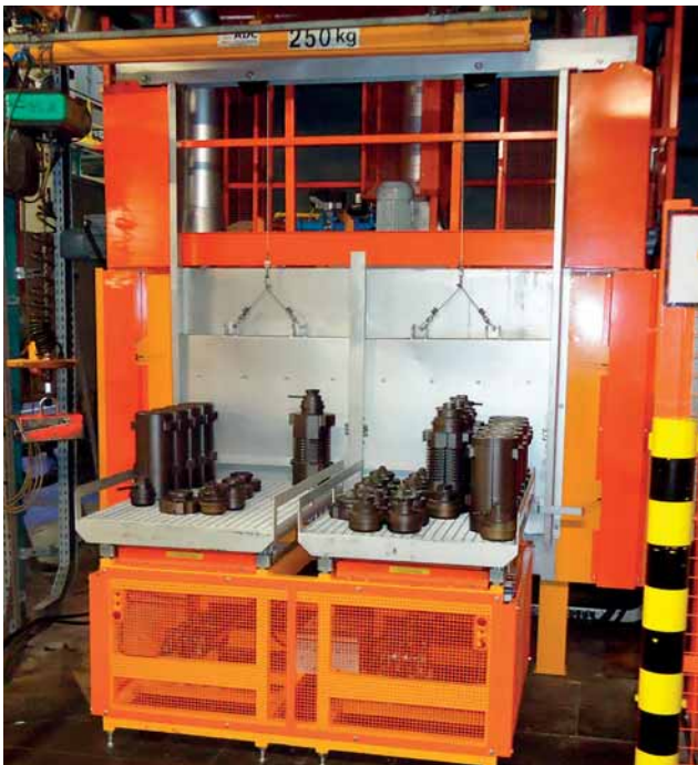
MOLDS PRE-HEATING OVEN
