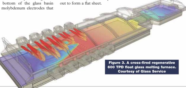
this technology be installed in a conventional regenerative float furnace converted to oxy-gas firing, a total of 20-25 percent energy savings may be achieved. A side effect would be a major NOx reduction.
