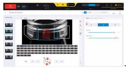
← At a pace of 350 BPM, Saturn can analyze up to 792 high-resolution images to catch the tiniest checks on bottles and jars. Production quality is kept at the highest level while any false reject level is significantly reduced. Resorting -often caused by checks defects- can also be reduced by up to 90 percent compared to standard technology.
