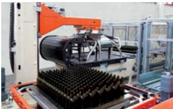
'MPH' Multi-Purpose Palletizing Head
