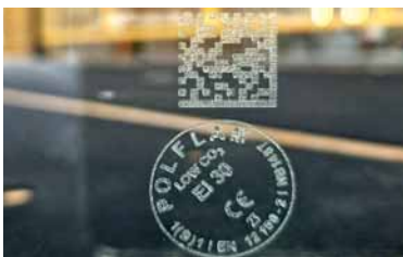
POLFLAM GAIA low-carbon fire-resistant is recognisable by the LOW CO 2 product marking
