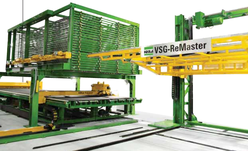
Linear Driven Cutting Machine for float glass: Hegla Galactic
