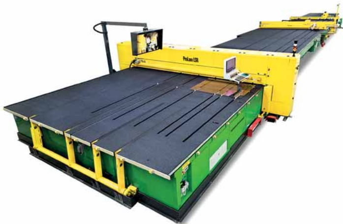
ProLam LSR: Improved productivity and edge quality thanks to laser diode heating technology
