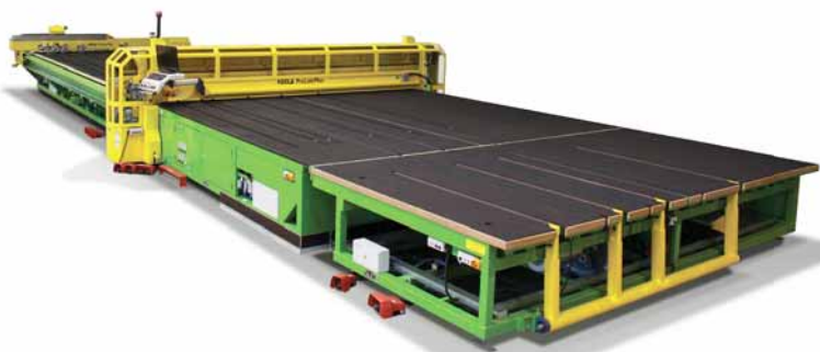
ProLam Plus Shape: Model cutting system for laminated glass
