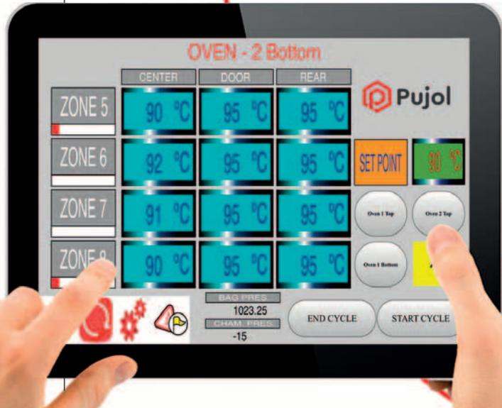
will be able to have greater control over what happens at all times with their furnaces, thus achieving greater comfort and greater peace of mind. Pujol e-Connect allows real-time access to the state of the furnace, with the possibility of programming parameters and, for greater peace of mind, receiving a notification of any incident that occurs during the laminating process. It includes,
