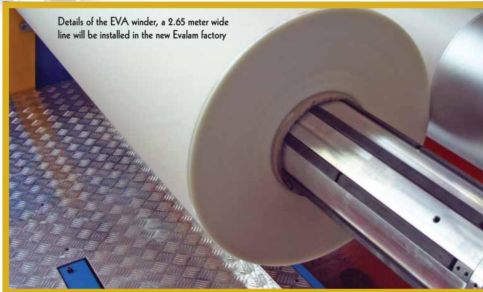
Details of the EVA winder, a 2.65 meter wide line will be installed in the new Evalam factory
