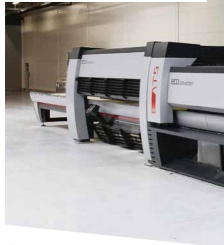
from 1500x3800mm to 3300x6000mm, and is also available in customizable sizes. The ATS 4.0 series hardens glass with the highest optical and flatness standards, thanks to
