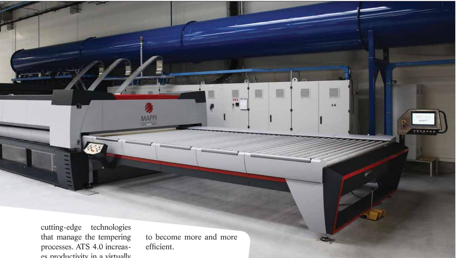
cutting-edge technologies that manage the tempering processes. ATS 4.0 increases productivity in a virtually continuous cycle with no downtime for the regulation of operating temperatures and most of the operating parameters.
