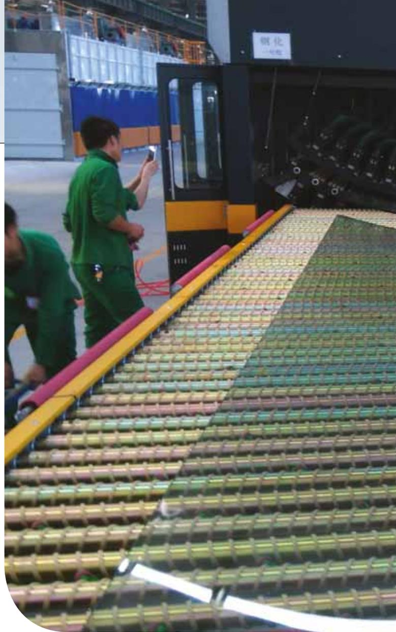
be bent. After heating, the glass is loaded and shaped on pre-set bending sections at the same time.
