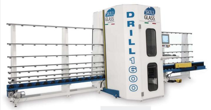
ness of 3-20 millimetres. The machine is composed of five axes, X Y V Z W, and two electro-spindles which, as opposite drilling heads, create a double-sided drilling system that drills perfect holes.
