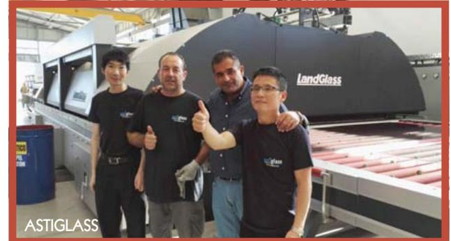
ny's clean, spacious workshop, the Cyclone series glass tempering furnace can immediately be seen, and features a revolutionary arc-shaped structure, and the new generation Cyclone™ Convection heating system. Through the optimized design for the convection fans and enclosure, it offers better matched parameters and unprecedented uniformity of convection air pressure
