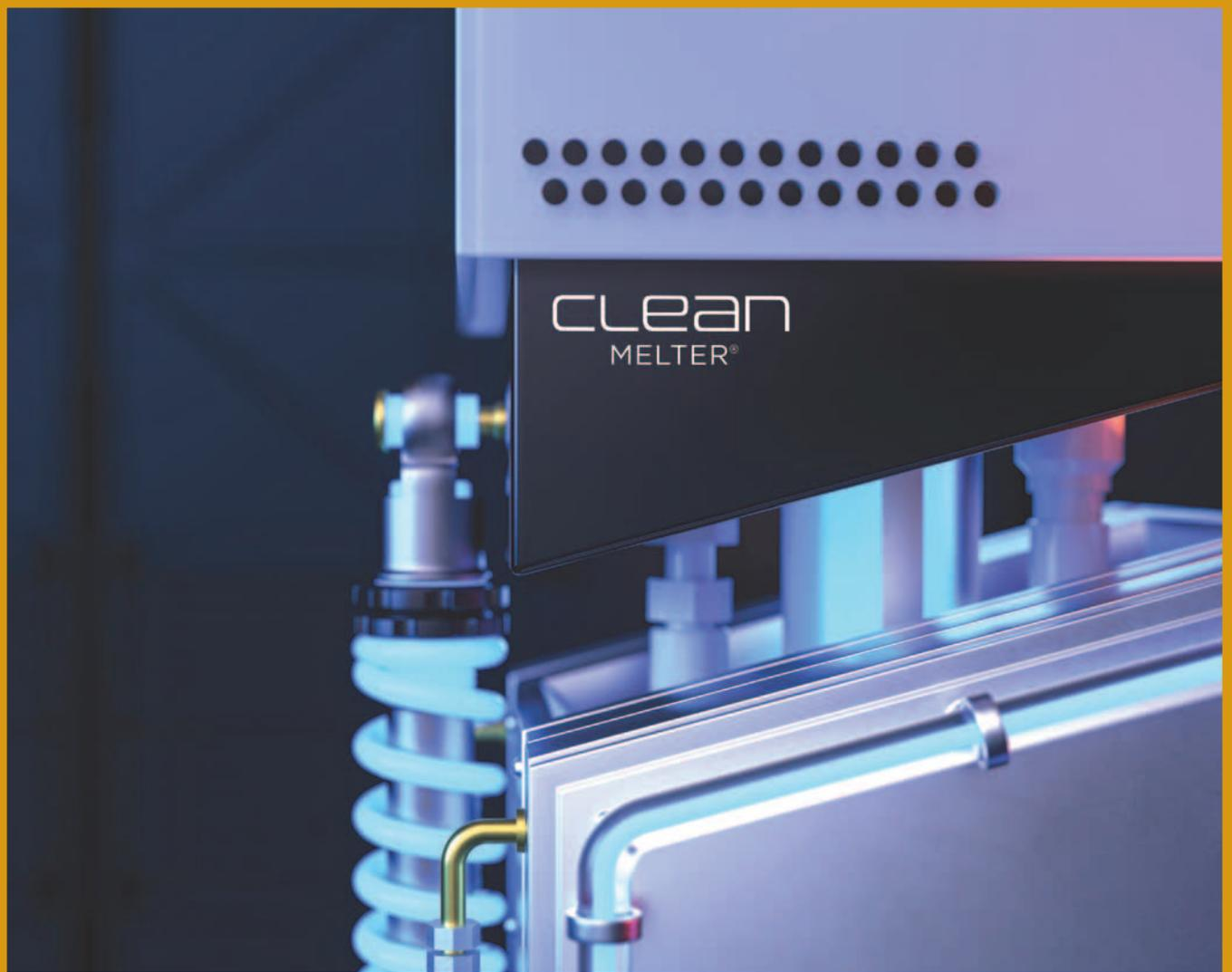
energy consumption and carbon emissions, while also offering huge cost savings and greater flexibility in terms of pull variations, raw materials and raw material changes – all without affecting glass quality. The furnace's refining shelf stabilizes the melting process, with the increased glass temperature above reducing viscosity and releasing all blisters on the surface. With decades of refining shelf experience, SORG knows that without it, the required quality of glass is not achievable.
