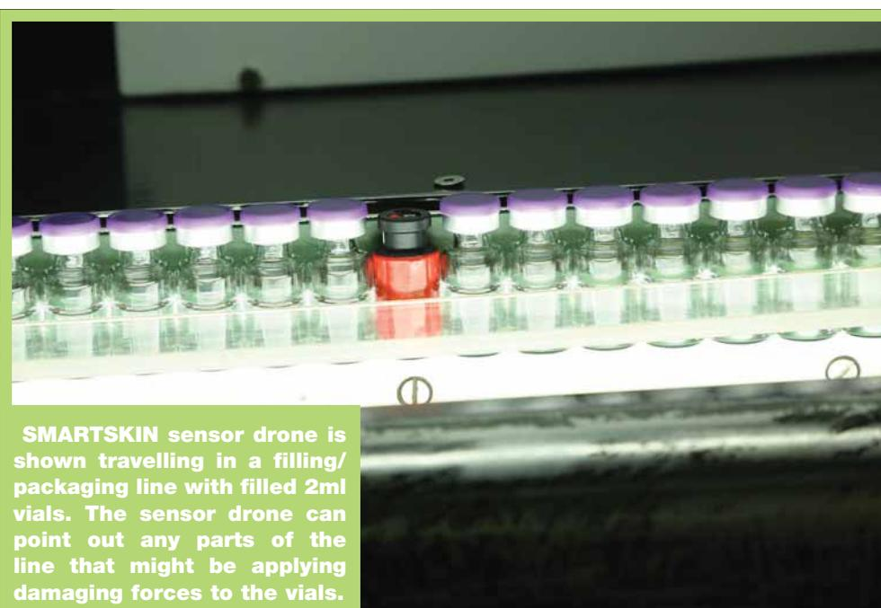
**SMARTSKIN sensor drone is shown travelling in a filling/packaging line with filled 2ml vials. The sensor drone can point out any parts of the line that might be applying damaging forces to the vials.**
