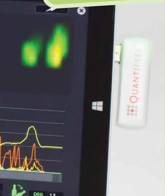
Two SMARTSKIN replica vials (sensor drones) are shown alongside a tablet showing the Quantifeel™ software. The software shows the pressure points measured on the sidewall of a drone, as well as other data streams such as shock, tilt and rotation.
