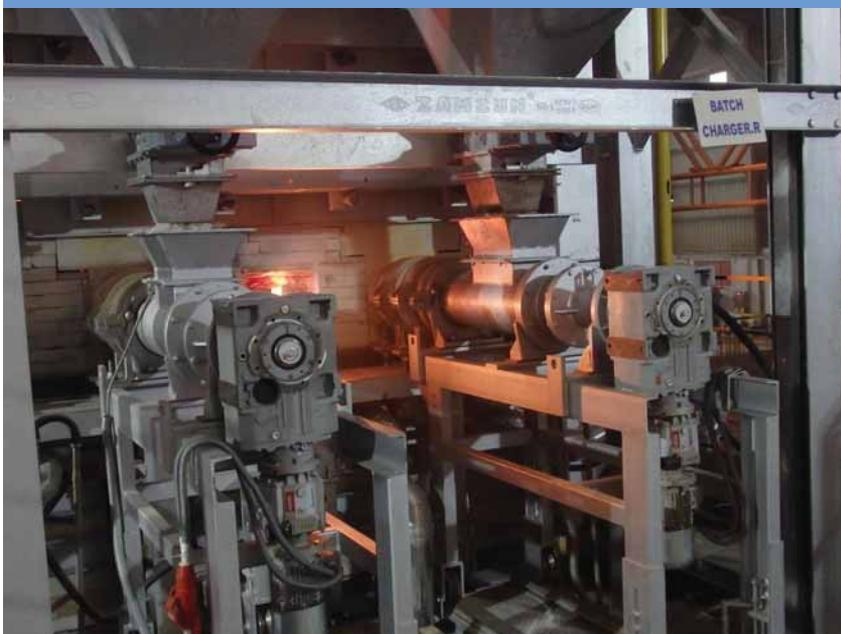
Achieving this level of performance requires accurately engineered: refractory design, burner design and positioning, booster electrode position, water cooled bubbler tubes, temperature management, special throat cooling technology, and special side cooling technology. After a four-year run, 65 per cent of AZS and refractory materials should be changed, while the steel structure and equipment can be used for a second run.
