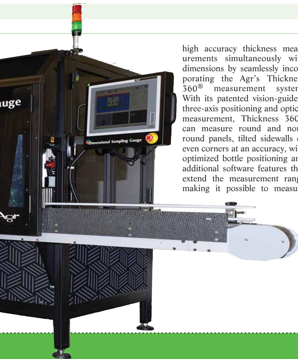
high accuracy thickness measurements simultaneously with dimensions by seamlessly incorporating the Agr's Thickness 360® measurement system. With its patented vision-guided, three-axis positioning and optical measurement, Thickness 360® can measure round and non-round panels, tilted sidewalls or even corners at an accuracy, with optimized bottle positioning and additional software features that extend the measurement range making it possible to measure
