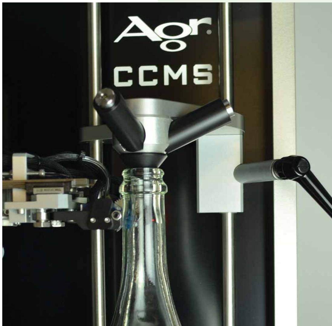
Close proximity to production improves testing efficiency and makes it practical to perform volume and fill-level measurement, more often, on a regular and timely basis. As a result, plant operators are able to closely measure volume and fill level with high precision, on a regularly scheduled basis throughout the production run, making it possible to better manage and meet customer quality requirements.
