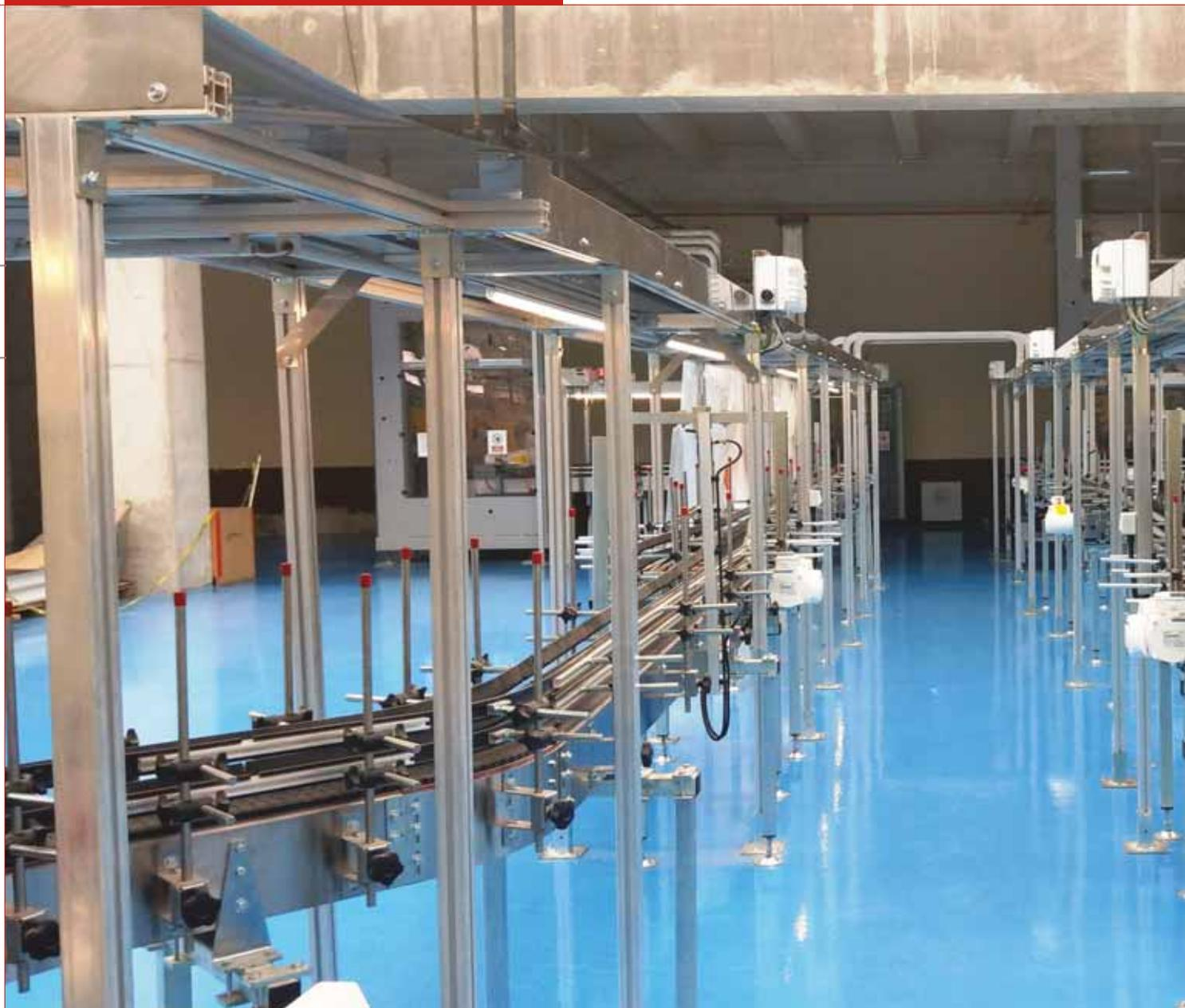
conveying and palletizing lines for empty glass articles (namely bottles and jars).
