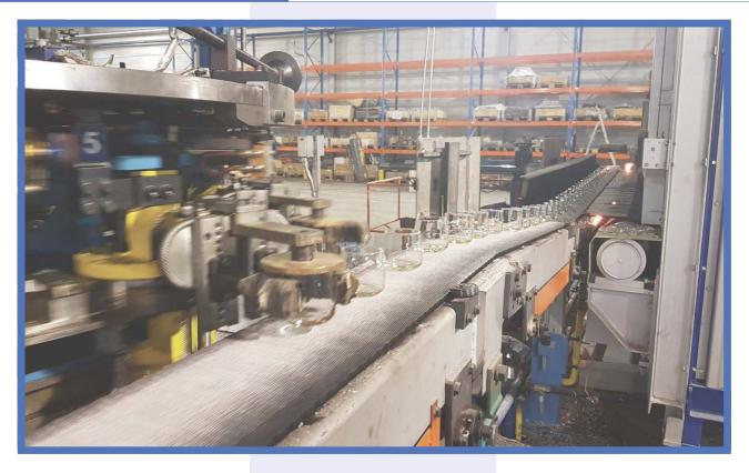
a purely mechanical machine. There are a great number of H28 machines still up and running around the world and the only reason for substituting them is based on the more modern 'electronic' method of working that we have now.
