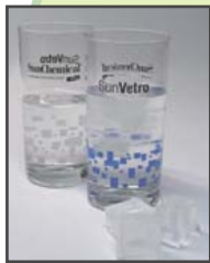
Figure 1 - Thermochromic inks were applied to these glasses. Colder temperatures change the colour of the ink from white to blue
