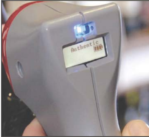
Figure 3 - Sun Chemical's Verigard™ security product is a proprietary machine-readable covert taggant system used to protect some of the world's most recognized consumer products from counterfeiting and diversion. Samples of glass decorating that used Sun Chemical's inks and coatings
